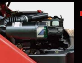
► The new stamped air cleaner featuring tangential intake, double seal with safety filter is durable, corrosion-free and vibration-resistant, provides better filter efficiency and lower intake resistance than the previous.
